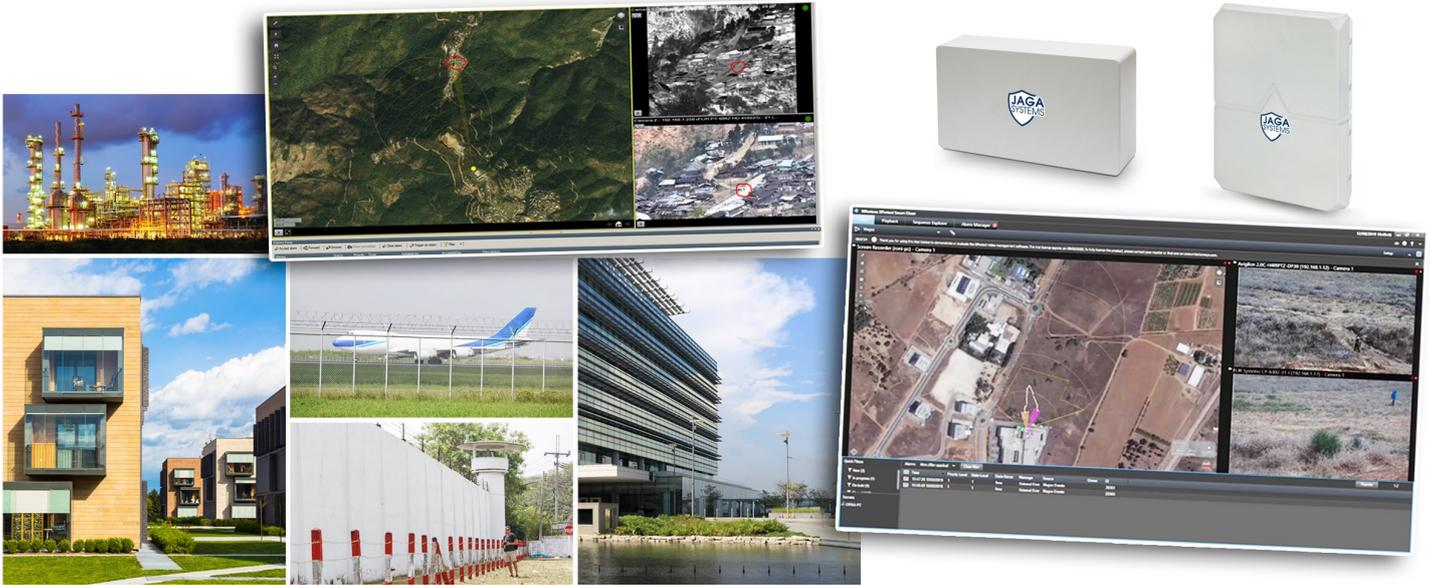
Jaga Systems solution is a compact and robust radar that provides complete situational awareness; with volumetric detection. Using cutting edge sensing technologies to prevent intrusions. Single unit detects movement upto 1000m in 120° band.
